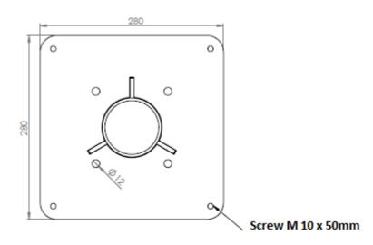
For unbounded subbase use the additional installation tool and insert them in a fresh concrete bed C 12/15. After curing process screw them together with the base plate.
